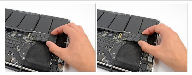
• Slightly lift the rightmost side of the SSD and firmly slide it straight away out of its socket on the logic board.
